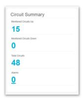
The Circuit summary card displays the current counts for the Circuits in inventory along with basic monitoring information and the Alarm count data for any monitored circuits
