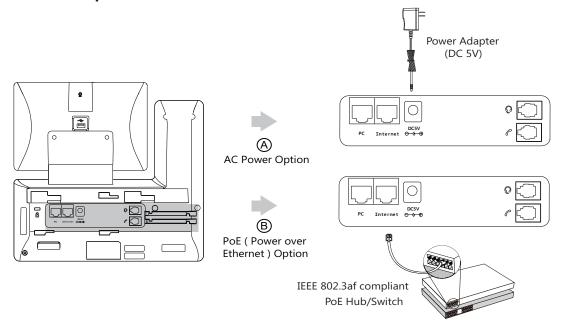
Note: The IP phone should be used with Yealink original power adapter (5V/2A) only. The use of the third-party power adapter may cause the damage to the phone.
