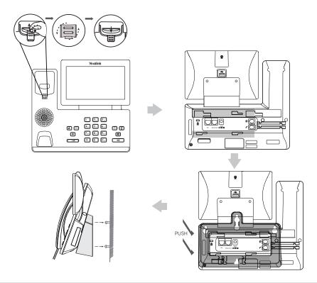
Note: The hookswitch tab has a lip which allows the handset to stay on-hook when the IP phone is mounted vertically. For more information, refer to Yealink Wall Mount Quick Installation Guide for Yealink IP Phones.
