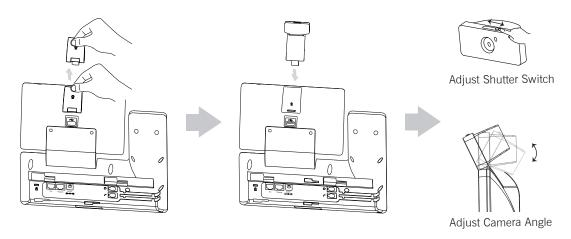
Note: The camera can only be connected to the USB port on the top of the phone. And the IP phone only supports the Yealink original USB camera CAM50.
