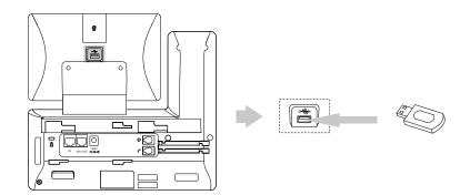
Note: The USB port (on the rear of the phone) can also be used to connect color-screen expansion module EXP50 or USB headset. For more information on how to use EXP50, refer to Yealink EXP50 User Guide. For more information on how to use USB headset, refer to the documentation from the manufacturer.
