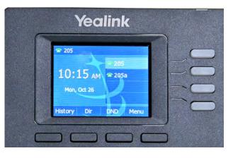
The keys to the right of the screen are programmable Line Keys. Each can be set per the configuration of the phone and/or configured as speed dials or 'favorites'. In the example above, there are two line keys that have been configured on the top two buttons.
