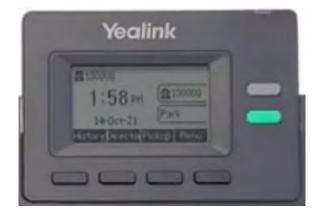
The two keys to the right of the screen are programmable Line Keys. Each can be set per the configuration of the phone and/or configured as speed dials or 'favorites'. In the example above, both line keys have been configured.
