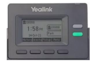
The two keys to the right of the screen are programmable Line Keys. Each can be set per the configuration of the phone and/or configured as speed dials or 'favorites'. In the example above, both line keys have been configured.
