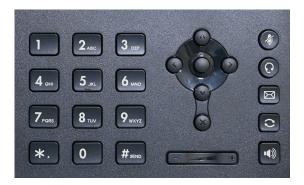
The four-way navigation pad allows the user to move through the phone's menu system and make selections, and the four arrow keys also double as shortcuts. Pressing UP displays the call history, pressing DOWN displays the number directory, LEFT and RIGHT select the line appearance key to use for making an outgoing call.
