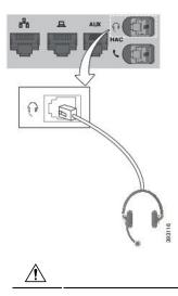
**Caution** Failure to press the cable into the channel in the phone can damage the printed circuit board inside the phone. The cable channel reduces the strain on the connector and the printed circuit board.
